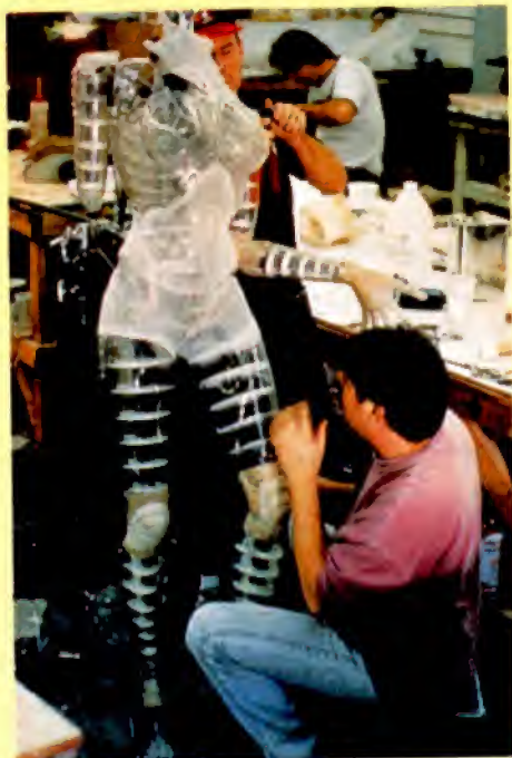
XFX technicians Eric Feldler (l) and Bob Newton construct the transparent animatronic Sil puppet.
